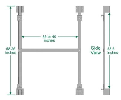
**Diversimount** employs a unique system of two uprights with a cross member and 5 lower mounting positions with variable length slots at top truly making it a "one size fits all" solution! **Diversimount** also borrows some key design elements from our flagship track mount system, **Diversitrack**. Namely our flexible clip system that holds tight to your favorite interactive white board.
